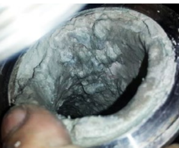
Before Vulcan was installed the filter was full of hard limescale deposits.
