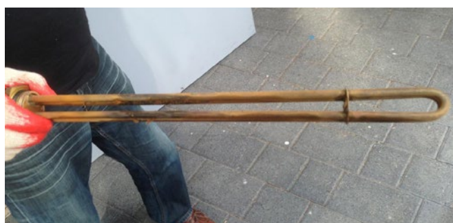
Scale deposits completely removed after 3 months
