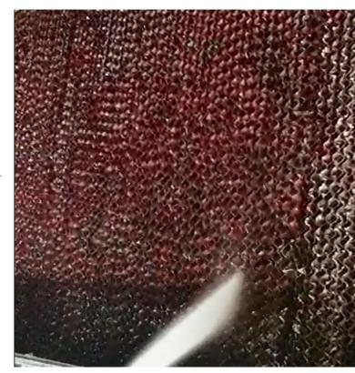
After Vulcan S10 had been installed for 2 weeks, the old scale had been softer, and the new scale had formed as powder. The new scale was easy to clean, and the old scale took more time to clean up with a water gun.
