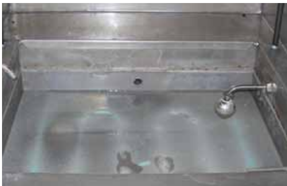
Before Vulcan installation - scale deposits found on Pan surface.
